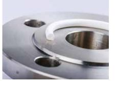
KWO® Universal Tape R is a round sealing cord, which is manufactured with the same technology than the KWO<sup>®</sup> Universal Tape F Premium. The round shape has no additional adhesives and is suitable for high purity applications, where the gasket is positioned in the respective wells provided.
